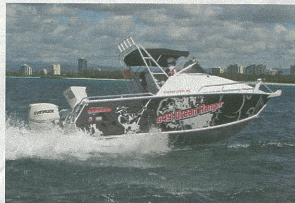
The 649 Ocean Ranger is Stacer's first foray into offshore plate boats. It offers plenty of space, a deep-vee hull and loads of storage.
