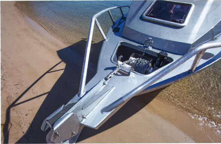
Everything on the Stacer is built to withstand hard work. The big drum winch is easily accessed through the cabin hatch, while the anchor rests on a sturdy bowsprit.
