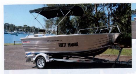
The Stacer 449 Northern Fisher comes standard with a 70-litre fuel tank, which is relatively generous for a boat this size. Interestingly, it's the same fuel tank they put in the bigger model boat.
