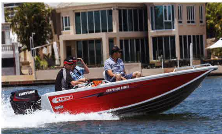
Keen observers might see subtle differences in the hull shape of the 429 Proline Angler. Chines have been widened and the bow entry is sharper in the 2016 models.
