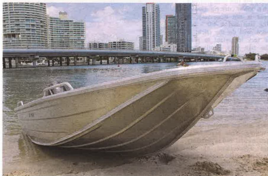
One difference in the Striker Series is that the chines no longer meet in the centre line, providing better stability.
