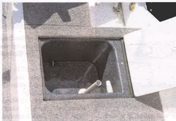
One option sure to be selected by prospective Proline 449 Angler owners would be the live well, in this case a roto moulded job.
