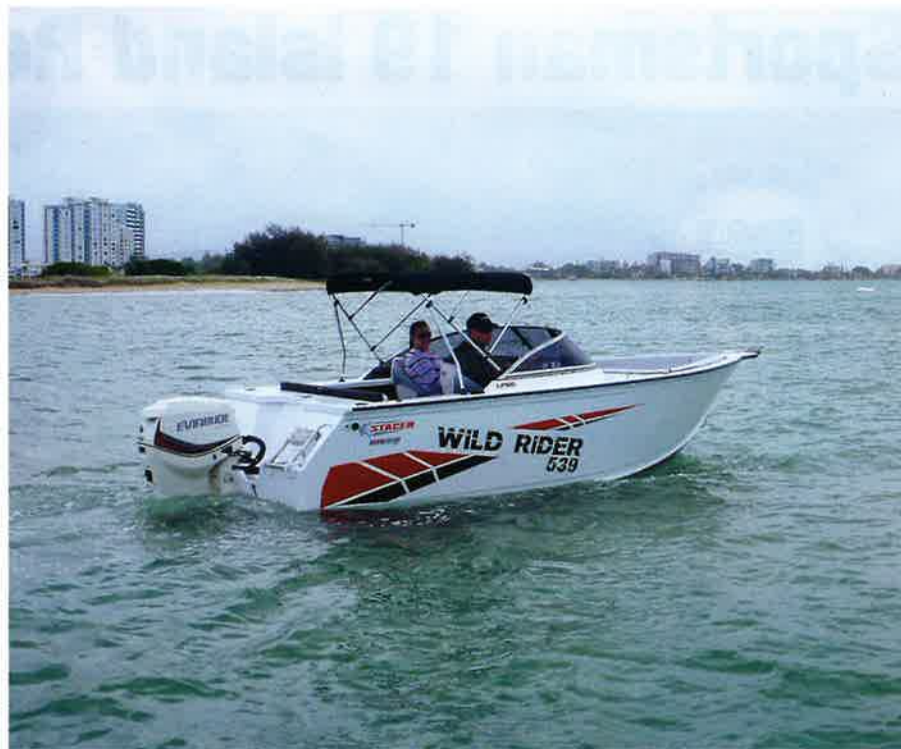
Many of the features in Stacer's 2018 range can be seen in this shot of the Wild Rider 539 at rest. Note the full height transom, high sides offering plenty of freeboard, and the great proportions of this rig as a whole.
